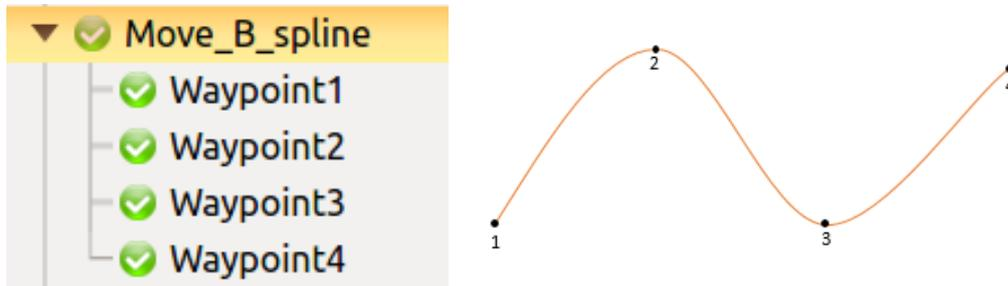
Figure 11-21 B-spline curve
