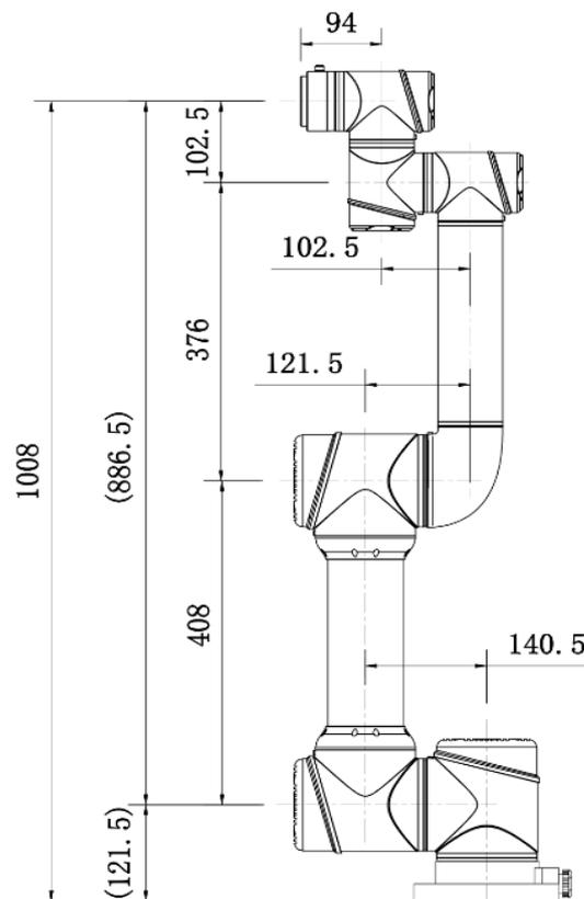
Figure 6-1 AUBO – i5 mechanical dimensions, unit: mm
