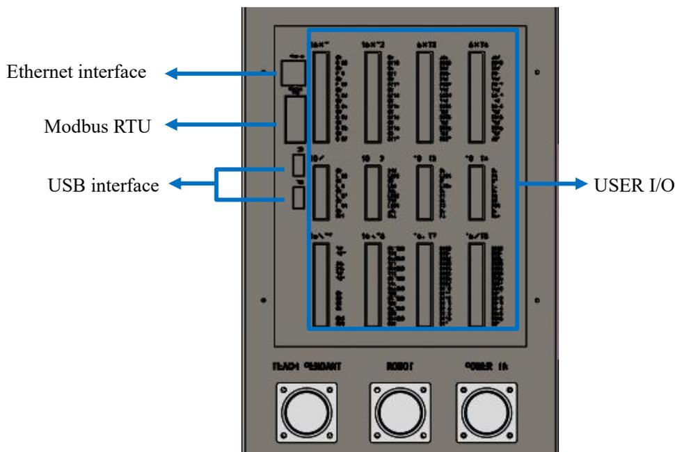
Figure 7-7 Communication interface on the back of the control box
