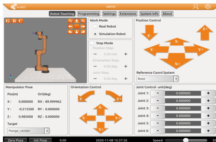
Figure 9-5 AUBOPE robot operating page (Simulation Mode)
