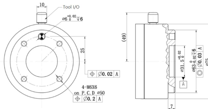
Figure 6-8 Mechanical dimensions of end-effector flange, unit: mm.
