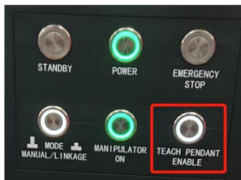
Figure 7-10 Control box panel
