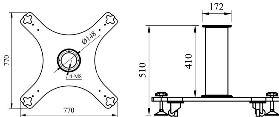
Figure 6-4 Mechanical dimensions of the manipulator base structure (left: plan view; right: front view)
