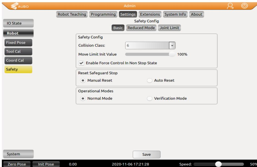
Figure 7-7 AUBOPE software “Setting” tag
