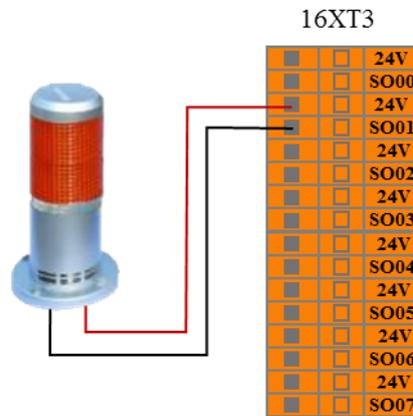
Figure 8-17 Figure robot moving output connection
