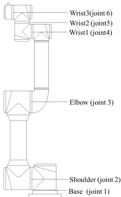
Figure 5-2 -1 Manipulator Joints
