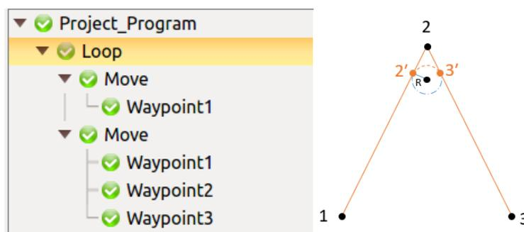
Figure 11-20 blending radius motion track
