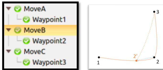
Figure 11-22 Arrival Ahead – Distance/Time Trajectory Example
