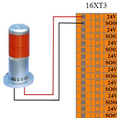
Figure 8-16 robot emergency stop output connection
